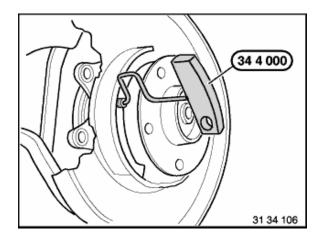
Twist clamping pin through 90° with special tool 34 4 000 and disconnect.
