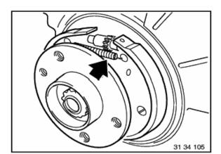
Disconnect return springs with brake spring pliers.
