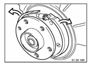
Spread brake shoes apart at bottom and lift off in upwards direction.
